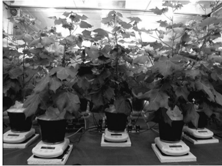
Figure 11. Five cotton plants on five balances in a growth chamber. This is what we call a mini-lysimeter system.
