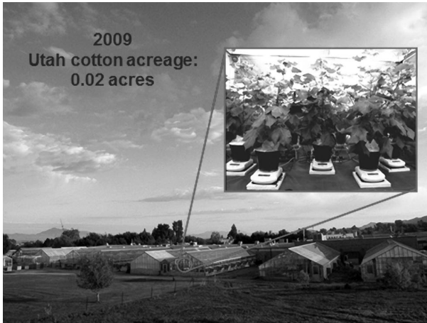
Figure 1. A photograph of the Utah State University Research Greenhouse complex. The inset shows cotton plants in electronic balances for studies on transpiration rate.
