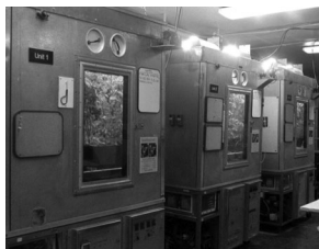
Figure 9. Three matching growth chambers at Utah State University that provide the equivalent of 80% of full sunlight at solar noon in the summer. Each chamber has been modified to include 4, 1000W high pressure sodium lamps and a recirculating, chilled water filter below the lamps. Cotton growth and development in this high light environment was excellent and representative of the field.
